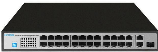
The PS12402FE-L is an unmanaged PoE switch with 24×10/100M PoE ports, 2× Gigabit RJ45 uplinks, and 1× Gigabit SFP port. All PoE ports support IEEE 802.3af/at up to 30W, with a total output of 300W. It auto-detects PoE devices to power APs, webcams, VoIP phones, and intercoms, ideal for hotels, campuses, factories, and SMEs.
