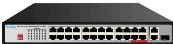
The PS12402FE Series Is An Unmanaged PoE Switch With 24 PoE Ports, 2 Gigabit RJ45 Uplinks, And 1 Gigabit SFP Port. Ports 1-20 Supply Up To 30W, Ports 21-24 Up To 60W, Max 300W Total. It Auto-Detects PoE Devices, Powering APs, Webcams, VoIP, And Intercoms, Ideal For Hotels, Campuses, Factories, And SMEs.
