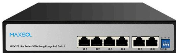
The PS1402E-L is an unmanaged PoE switch with 4×10/100M PoE ports and 2×10/100M uplink ports. Each PoE port supports IEEE 802.3af/at up to 30W, with 60W total output. It auto-detects PoE devices to power APs, webcams, VoIP, and intercoms, ideal for hotels, campuses, factories, and SMEs.
