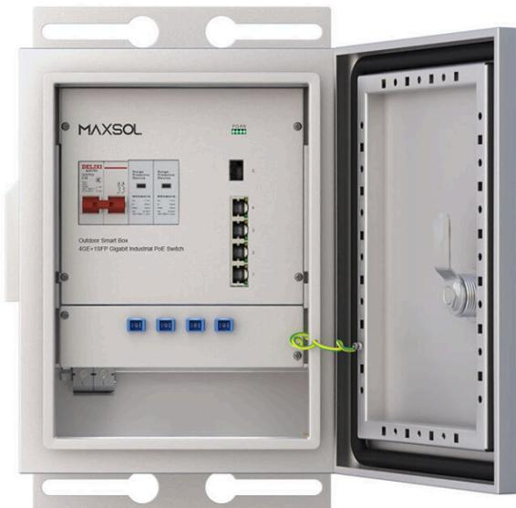
The SBOX2802SFGB-I-153WH is an outdoor industrial PoE switch with 8× Gigabit PoE ports (up to 2 supporting 90W PoE++) and 2× Gigabit SFP slots. Featuring full L2 functions, IP-rated and lightning protection, it operates from -40°C to 75°C. A built-in 153Wh LiFePO4 UPS ensures continuous power in harsh outdoor environments.
